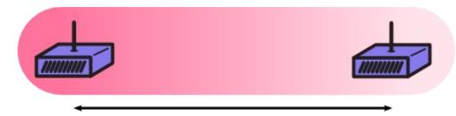
If the router moves too far away from the transmitter, it won't be able to receive any signal, either due to the signal being too weak or other signals interfering, and the routers will disconnect. Below we can see the two routers have disconnected, as there isn't enough signal.
