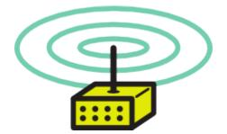
Using omnidirectional antennas has the benefit of creating connections in any direction. You don't have to do as much planning to connect with multiple neighbors or buildings. If there is enough signal between nodes, they should connect.
