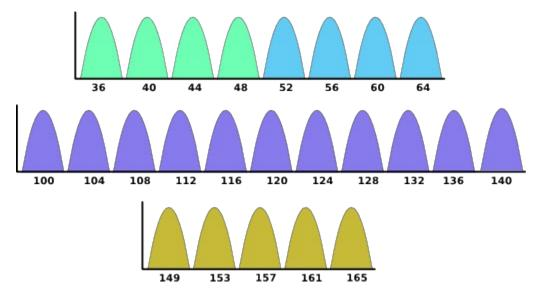
There are many more channels available in the 5GHz band, so it should be easier to select a channel in this band that doesn't cause interference. This may not always be true -- more and more wireless equipment is starting to use the 5GHz
