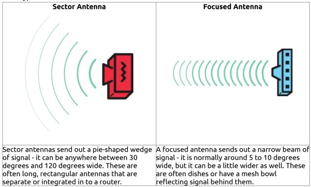
Using directional antennas has the benefit of increasing the distance a signal will travel in one direction, while reducing it in all other directions. Since the signal is all going one way, the power that would be sent out in all directions with omnidirectional nodes is now focused, increasing the power in that direction.
