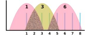
You could use other sets of Wi-Fi channels, as long as they are 5 channels apart - for instance 3, 8 and 13. This may not be optimal though, as channels 1 and 2 would be unused, and in many places in the world channel 13 is not available. Wherever you are, try and check what channels are most in use, and plan your network to use a channel that doesn't overlap.
